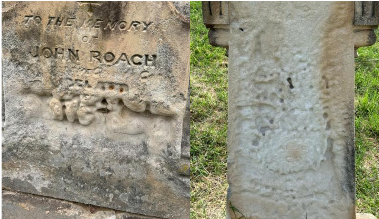
Figure 70: Weathering of sandstone (also known as honeycombing)
