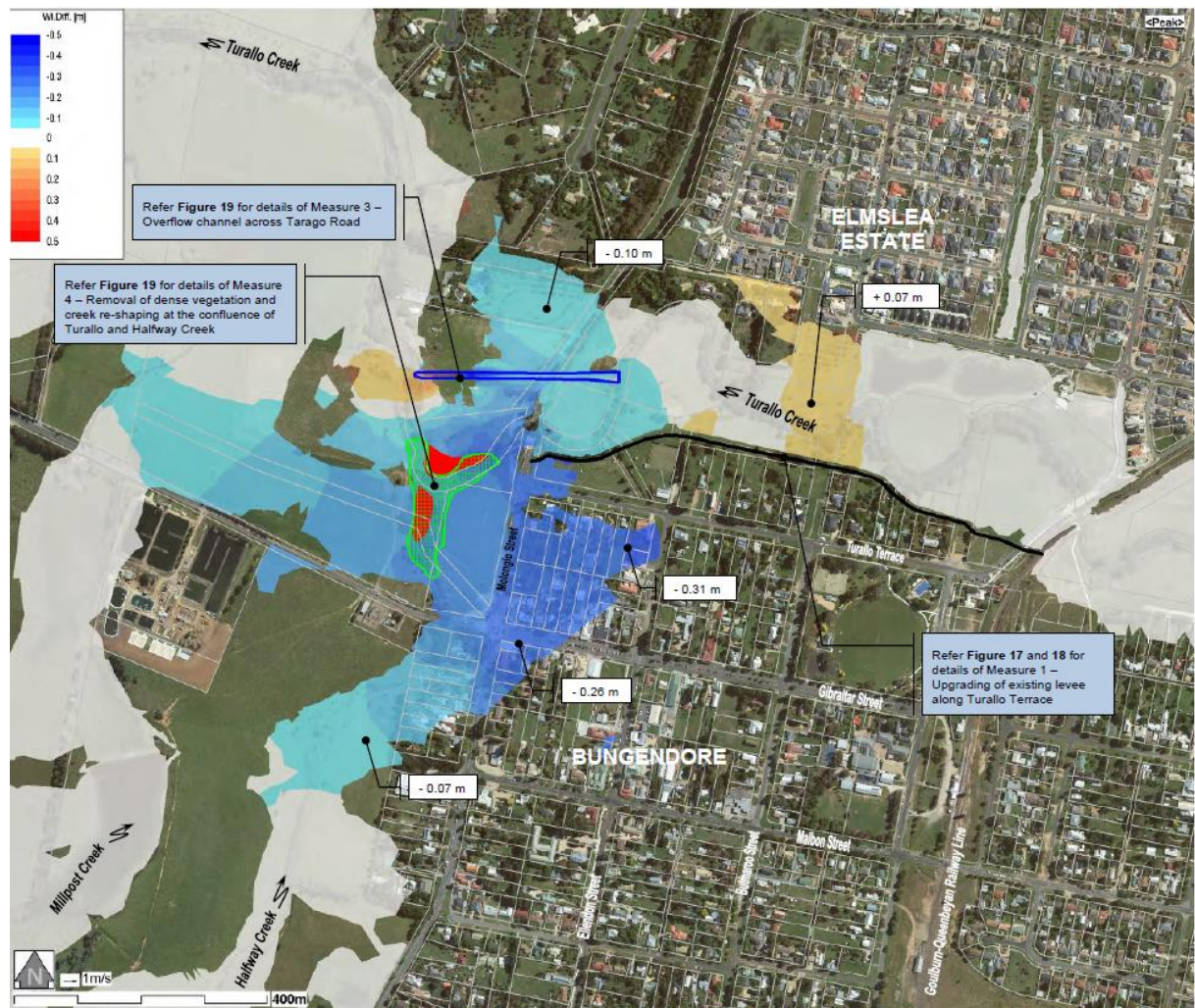
Figure 5-2 variation in peak 100 year recurrence flood levels due to the incorporation of Option S4B.
