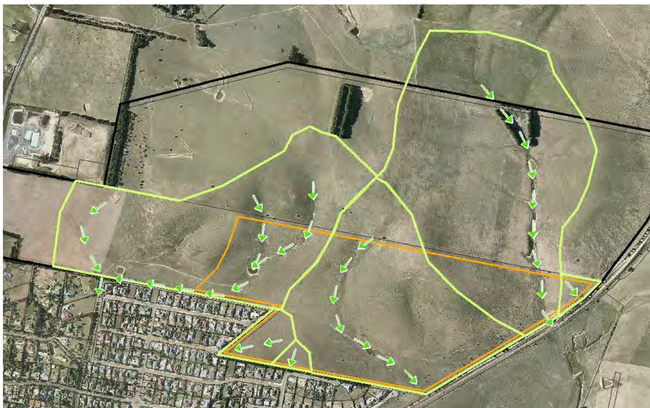
Figure 7-1: Planning proposal area stormwater outlet locations
