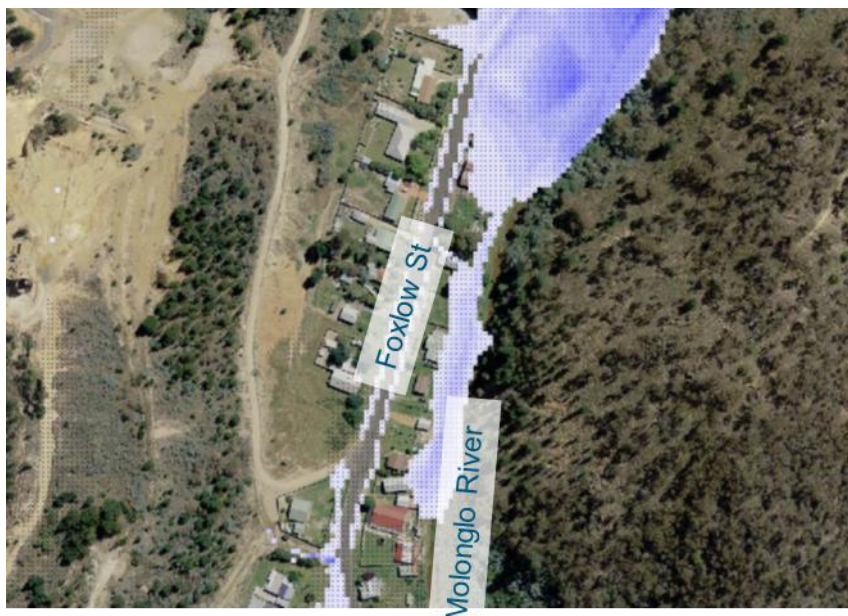
Figure 2-4 Inundation on the west bank of the Molonglo River near Captains Flat Dam (20% AEP event shown)
