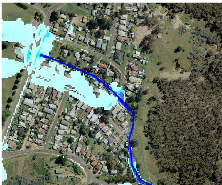
Figure 2-5 Flooding along Kerrs Creek (20% AEP event shown)
