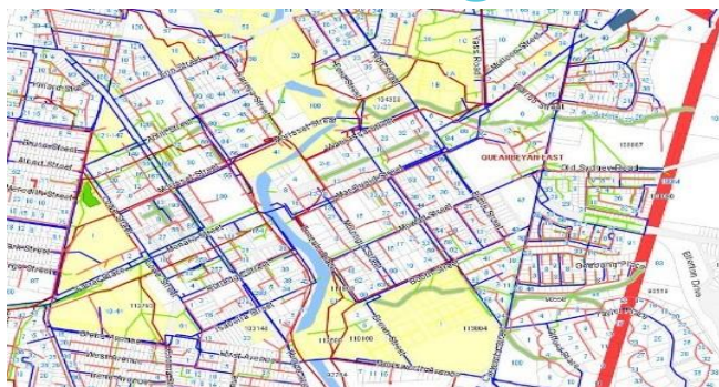
Water and Sewer Infrastructure in Queanbeyan.
